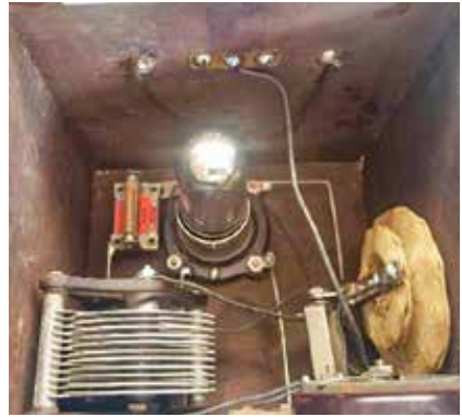
Right: Coil closed – maximum regeneration for a weak signal
