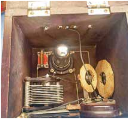
Left: Coil open – minimum regeneration for a strong signal
