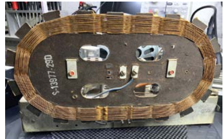
Figure 14. Rear of unit, case removed, showing AM antenna.
