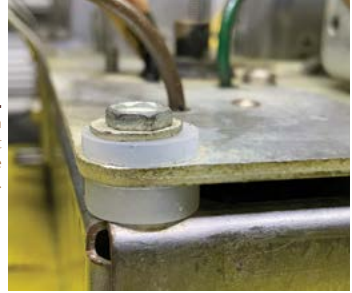
Figure 25. Speaker with replacement silicone grommets.
