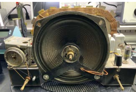
Figure 13. Front of unit, case removed, showing 7.5" speaker.
