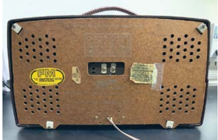
Figure 5. Back of unit showing no signs of water or other damage.
