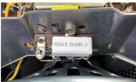
Figure 19. Replacement silicon diode and series resistor.
