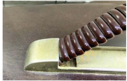
Figure 9. Top pitting and handle showing oxidation.
