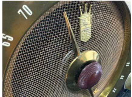
Figure 32. Close-up of grill, central control, and dial.
