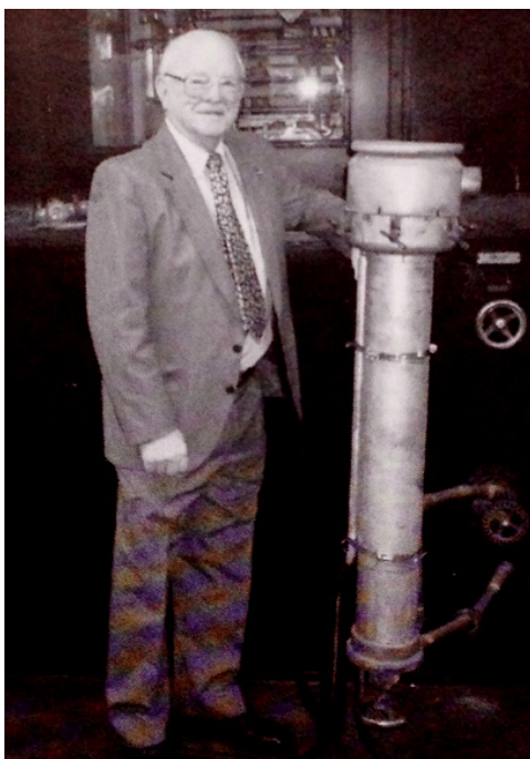
Charlie Stinger Standing By One of the Tube Sockets for the 898 Final Amplifier Tube Section of Crosley's 500 Kw Transmitter at WLW.
