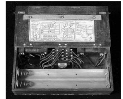
Inside the type SCR-57, BC-10 Radio Interphone Box.
