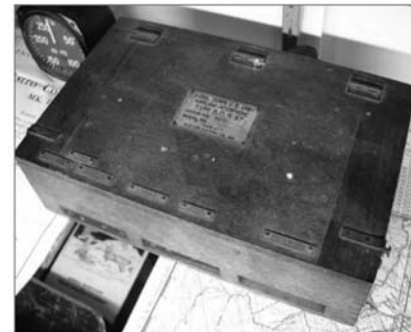
Type SCR 57, BC-10 Interphone Box on Display at the Hamilton Field Museum CA.
