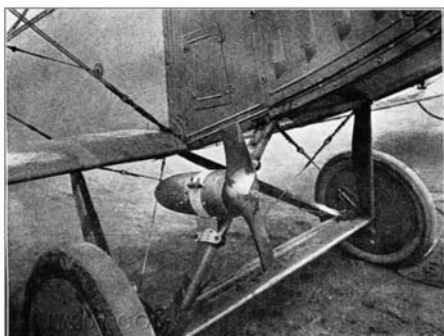
GN-1 Generator Installed on a Jenny.
