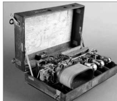
Inside the Type SCR-68, BC-11, Radio Receiver/Transmitter.
