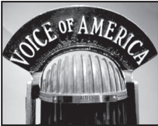
Voice of America microphone flag circa 1950. Western Electric introduced the 639A unidirectional ribbon velocity microphone in 1939, and it was sold by Altec in 1940s and 1950s. (Courtesy Audio Engineering Society)
