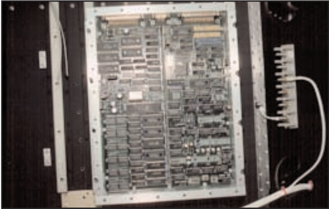
An early engineering model of Phase 3-D's Internal Housekeeping Unit (IHU).
