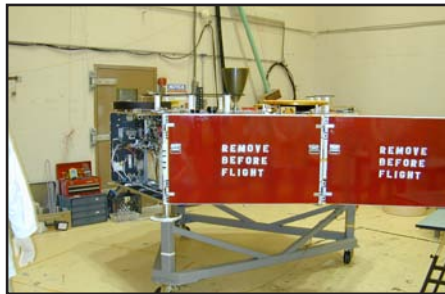
AMSAT’s Phase 3-D satellite is shown here during final integration. Note the “bar door” hinges on the solar panels.
