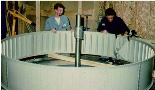
Students at Weber State University in Ogden, Utah work on the Specific Bearing Structure (SBS) for the Phase 3-D spacecraft.
