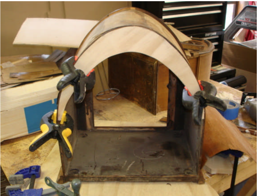
The replacement arch is now firmly attached to the top of the cabinet, using tiny nails through the sub-veneer.
