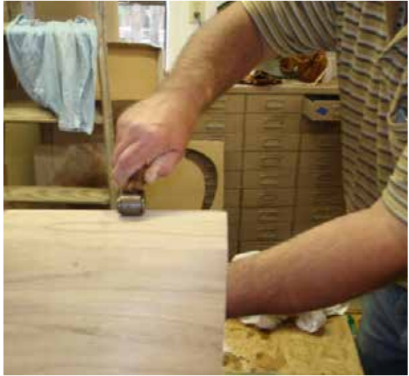
Rolling the veneer to eliminate air bubbles between the glue and the veneer and ensure a tight bond.
