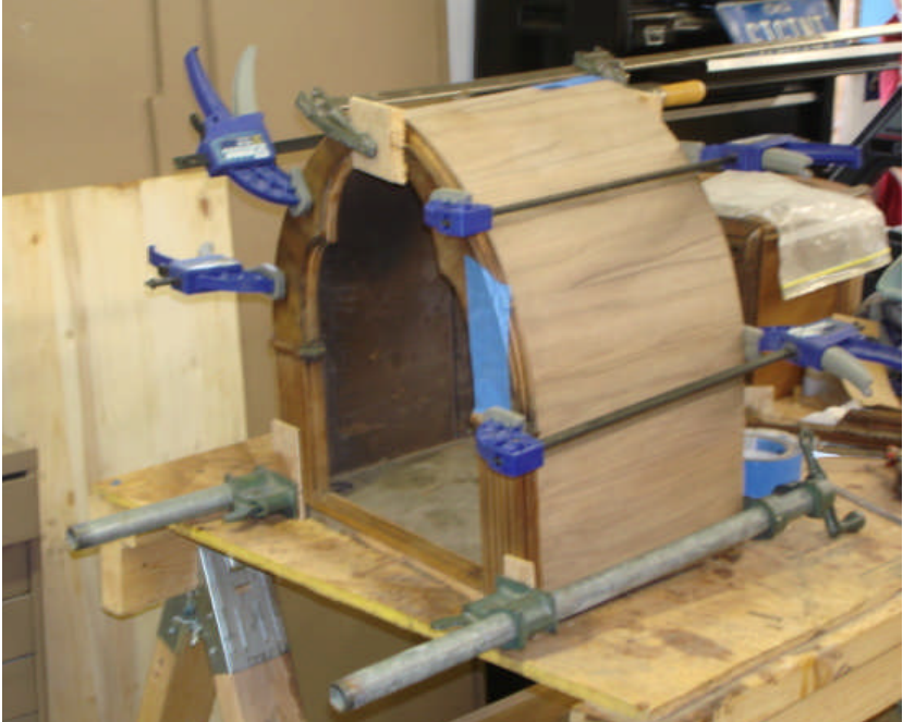
Reattaching the front. For this operation, lots of clamps are required.
