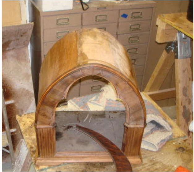
The arch at the top rear of this Philco 90 cabinet needed to be replaced.
