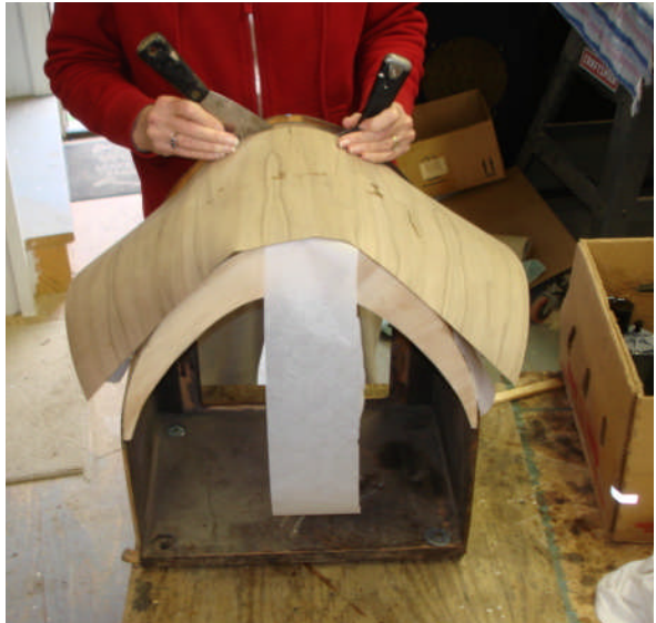
Here I am beginning to attach the new veneer to the top of the cabinet.
