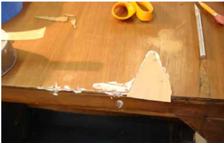
This Zenith cabinet needed veneer patches. Here I apply a piece of scrap veneer larger than the damaged area and then cut through both pieces with the Exacto knife..
