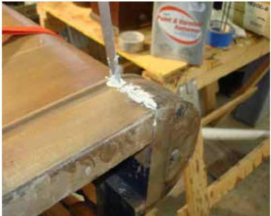
Securing a loose joint in the base of a cabinet. Force the glue/sawdust mixture in with a thin tool
