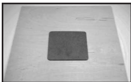
16 - The inner Masonite mold piece positioned on the base.
