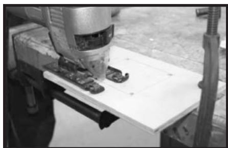
12 - Cutting out the mold with a saber saw.
