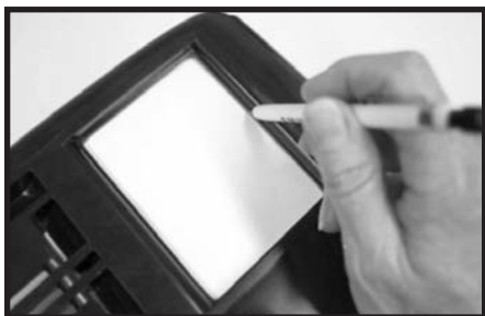
3 - Drawing the outline of the dial opening in a small Emerson Bakelite radio.
