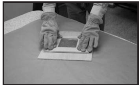
24 - Pressing the mold to form the plastic.
