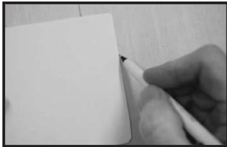
11 - Tracing the pattern onto a sheet of plywood to make a mold.
