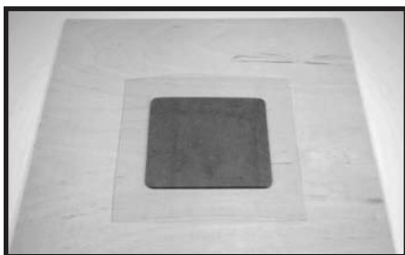
17 - The plastic centered on top of the inner mold.
