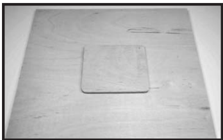
19 - The inner plywood mold piece positioned on the base.
