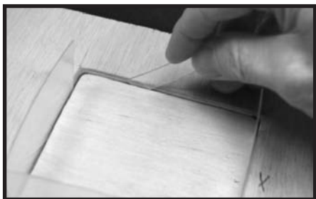
15 - Checking the mold halves for adequate clearance. (Extra large plastic pieces shown for clarity.)
