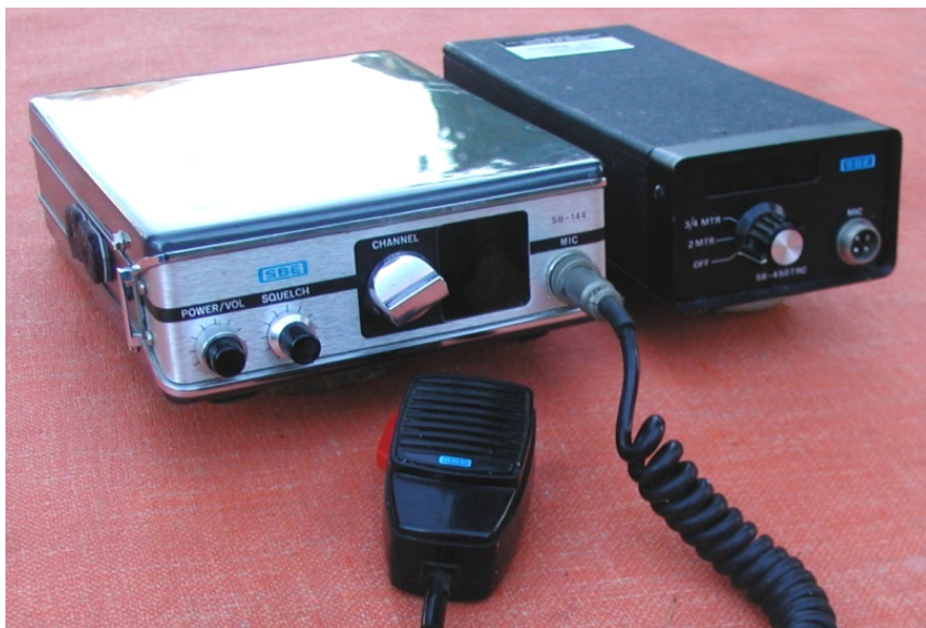
SBE's two meter (144-148 MHz) FM transceiver SB-144 (L) and TRC (R) adapter for UHF.
