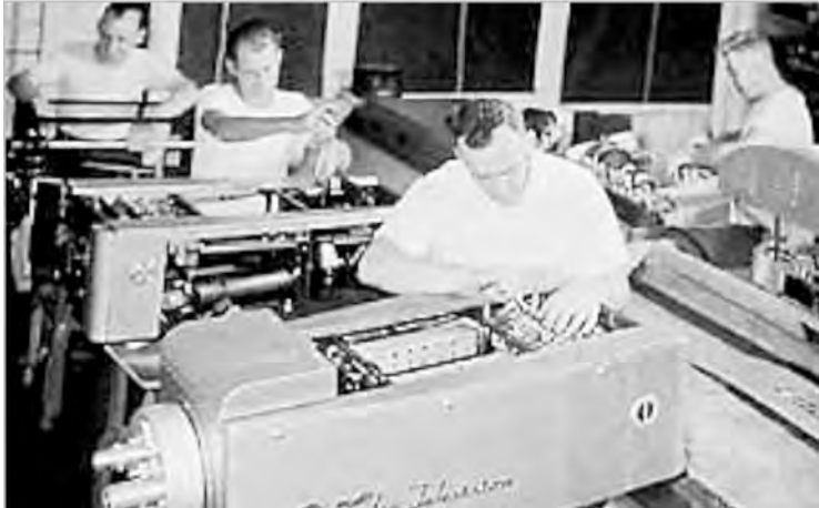
TK-40 assembly line, 1954. On the right rear of the camera body, the split, circular opening is an air vent for one of the image orthicon pickup tube. There are two additional vents on the rear of the camera.
