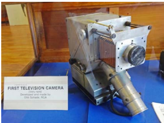
The very first RCA portable television camera at the new AWA Museum.
