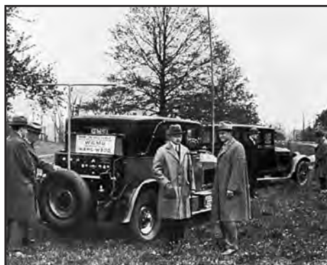
The A.H. Grebe Company's mobile station WGMU broadcast with 100 watts from a Lincoln sedan.
