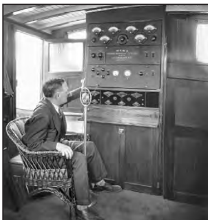
Maritime Mobile transmitter of the A.H. Grebe Station WRMU, 1926-27. The transmitter is at the top of the cabinet, a Grebe receiver is in the middle, and a motor generator is located behind the door at the bottom.
